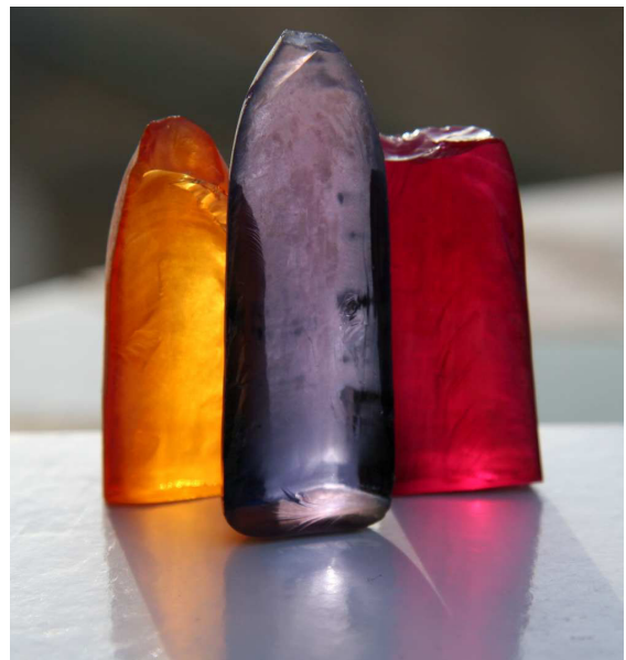
A selection synthetic sapphire boules, grown with the Verneuil method.
