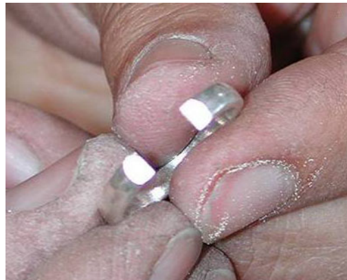
Ring shank after filing ends flat to properly fit the setting/
