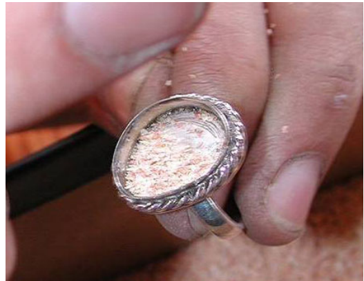
Sawdust is used in the setting to cushion the stone and align for the proper height of the stone in the setting.
