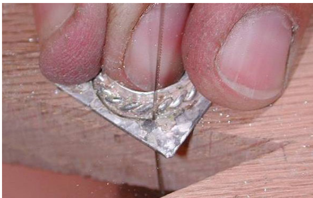
Trimming off the excess silver sheet from the base plate.
