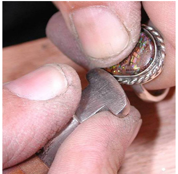
A bezel pusher is used to form the bezel around the stone.
