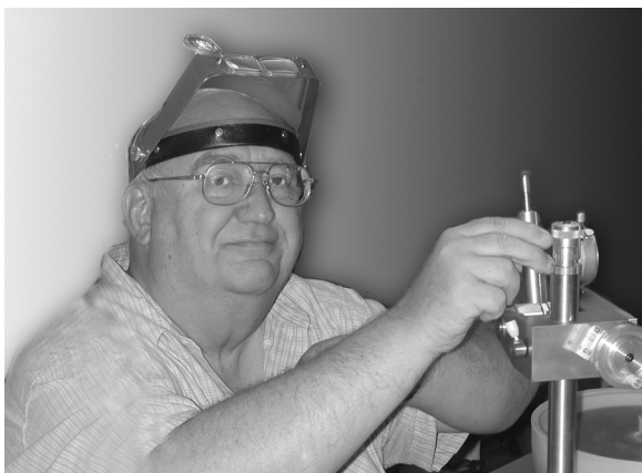
Facetor, Bill Wood is shown here finishing the polish of the crown on a large round synthetic ruby on his Facetron at the last workshop.
